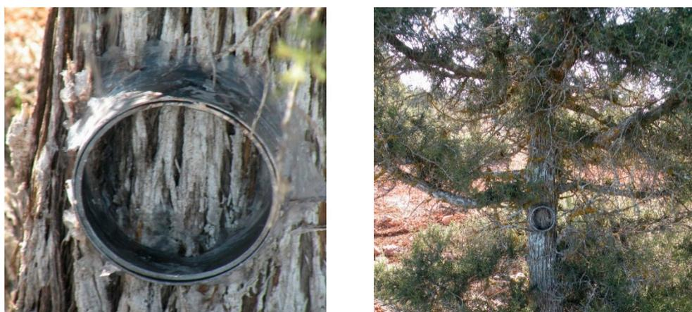
**Figure 3.** Metallic collar to measure stem CO<sub>2</sub> efflux in juniper trees in diameter at breast height.
