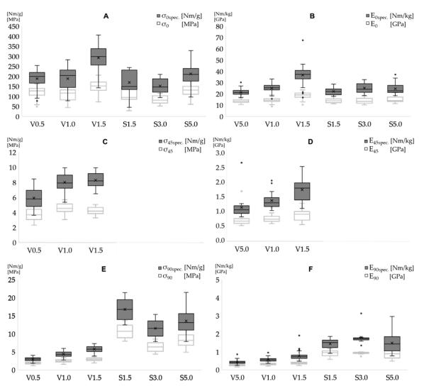
**Figure 2.** Boxplots of strength and stiffness as well as specific strength and stiffness for the respective thickness groups (V0.5, V1.0, V1.5, S1.5, S3.0 and S5.0): (**A**) strength at 0° load angle, (**B**) stiffness at 0° load angle, (**C**) strength at 45° load angle, (**D**) stiffness at 45° load angle, (**E**) strength at 90° load angle and (**F**) stiffness at 90° load angle.
