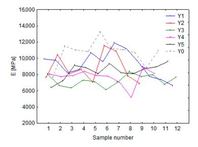
**Figure 6.** The radial variability of modulus of elasticity (MOE) of spruce wood depending on the period of time since the tree's decay.
