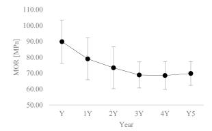
Figure 3. Resilience to static bending (MOR) of spruce wood in reference to the time since the tree's decay.
