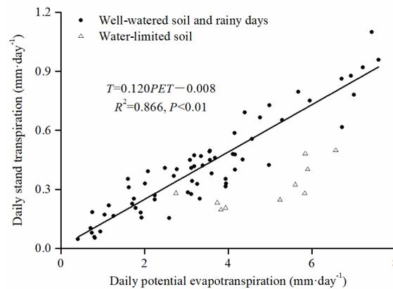
**Figure 5.** The relationship between the daily stand transpiration ( $T$ ) and daily potential evapotranspiration (PET) in the period of well-watered soil conditions and rainy days of 2015.
