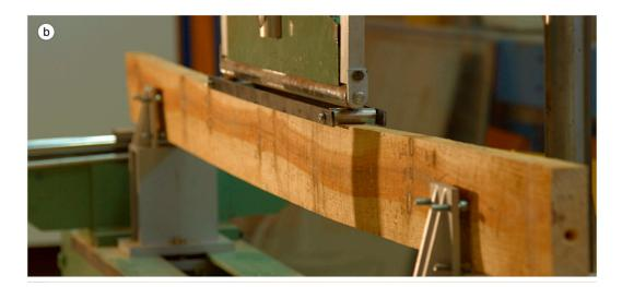
**Figure 4.** Bending test. (a) Diagram of EN 408 test [14] to determine modulus of elasticity (F: load applied, h: depth of cross-section, w: deformation); (b) piece under load.
