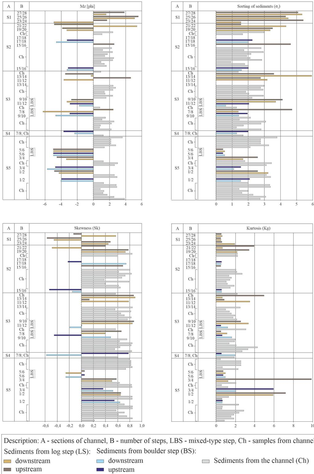
**Figure 7.** Variability of sedimentological indicator values in the longitudinal channel profile;- A—sections of channel; B—number of step; Mz—mean grain diameter,  $\sigma_1$ —sediment sorting, Sk—skewness, Kg—kurtosis.
