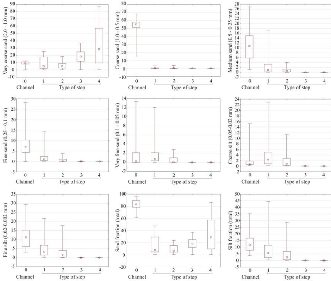
**Figure 5.** Differences between average values of standard deviations ( $\sigma$ ) of fraction of sediments sampled from 0—stream channel (Ch), 1—LS (upstream of log step), 2—LS (downstream of log step), 3—BS (upstream of boulder step) and 4—BS (downstream of boulder step).
