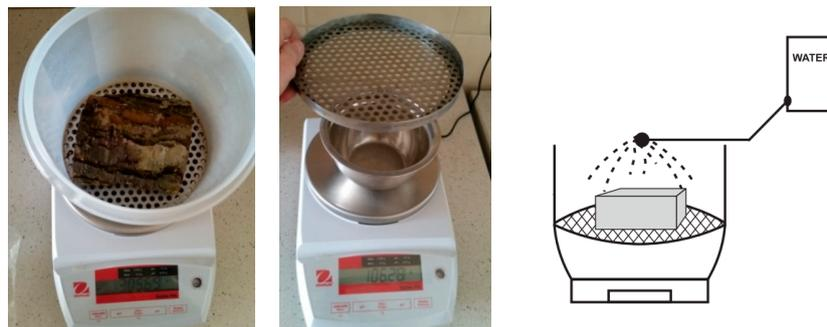
**Figure 1.** The water storage capacity measurement station and the analysis diagram.
