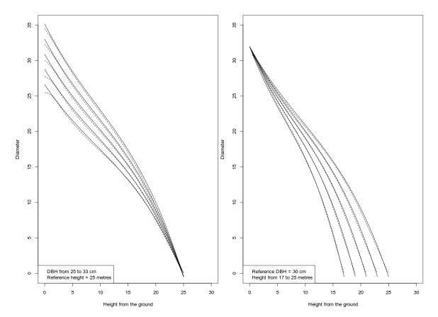
**Figure 4.** Stem profile generated using the third order polynomial function (continuous line) and TapeR package (dashed line) with two different hypothetical groups of *Pinus nigra* trees with same height but different DBH (left) and the opposite study case (i.e., same DBH but different height).
