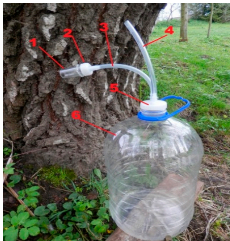
Figure 2. Tapping device components: (1) implant, (2) screw-on connector, (3) plastic tube, (4) plastic tube for air flow, (5) screw cap, and (6) container.
