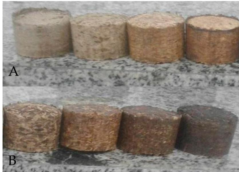
**Figure 1.** Briquettes produced at 10.34 MPa pressure. (A) = Briquettes produced from fresh biomass, left to right: bagasse, coffee, eucalyptus, and pine. (B) = Briquettes produced from torrefied biomass, from left to right: coffee, eucalyptus, pine, and sugarcane bagasse.
