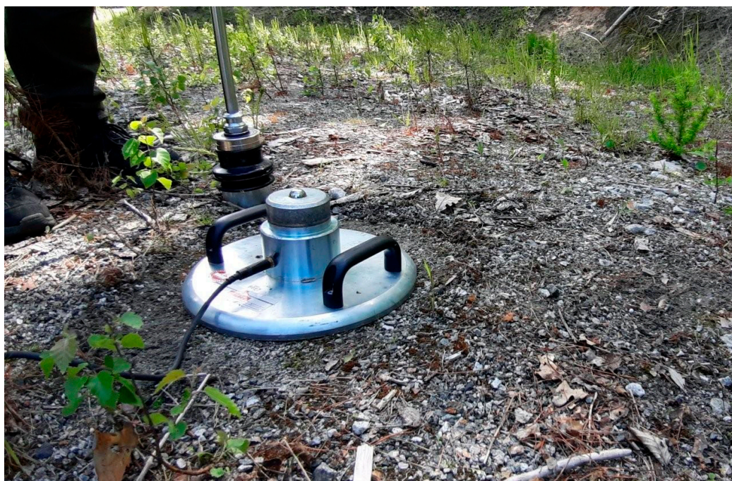
Figure 2. The bearing capacity testing with lightweight deflectometer on the experimental forest road section no. 2 in spring 2020, in the place where vegetation had been previously removed—“E” symbol in Table 2 (Photo: S. M. Grajewski).
