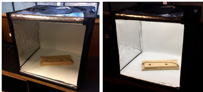
Figure 2. Photo studio lighting kit used to grade specimens.
