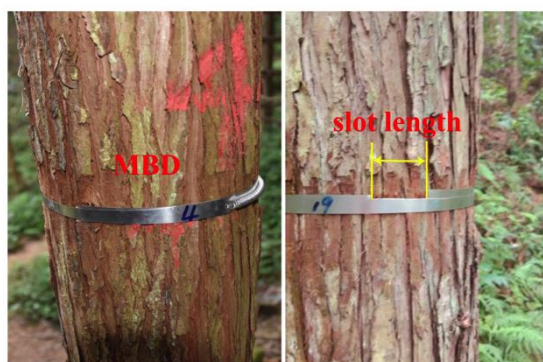
Figure 2. Manual band dendrometer (MBD) installed at breast diameter of Chinese fir.
