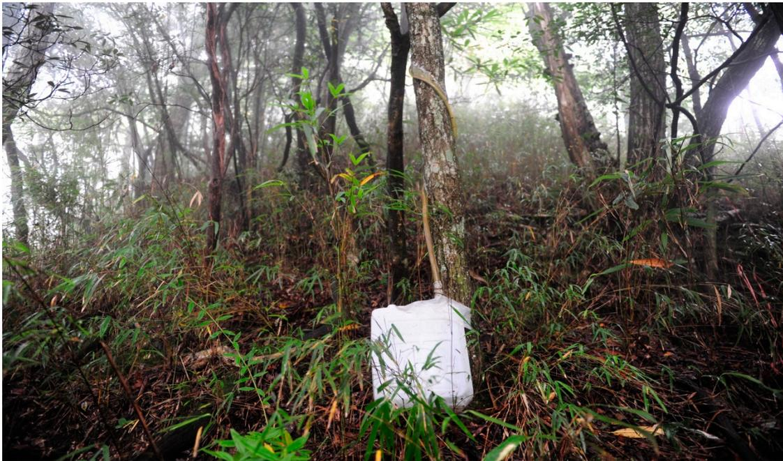
**Figure 2.** Stemflow collector with connected precipitation tank.
