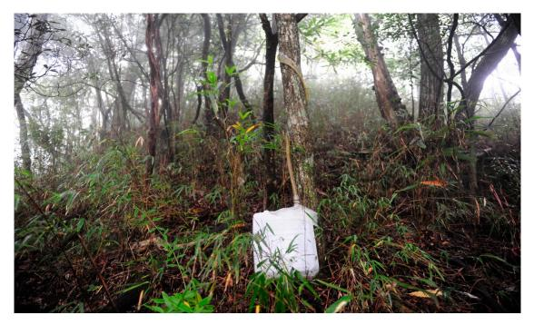
Figure 2. Stemflow collector with connected precipitation tank.
