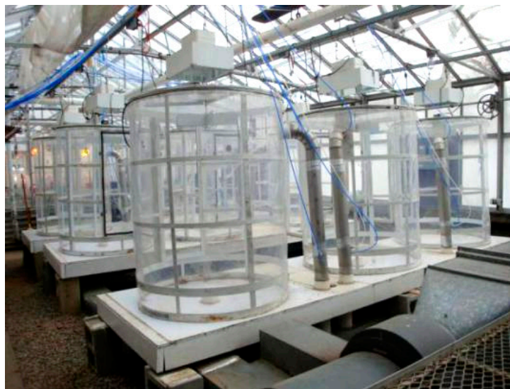
Figure 1. The nine continuously stirred tank reactor (CSTR) chambers in the experiment.
