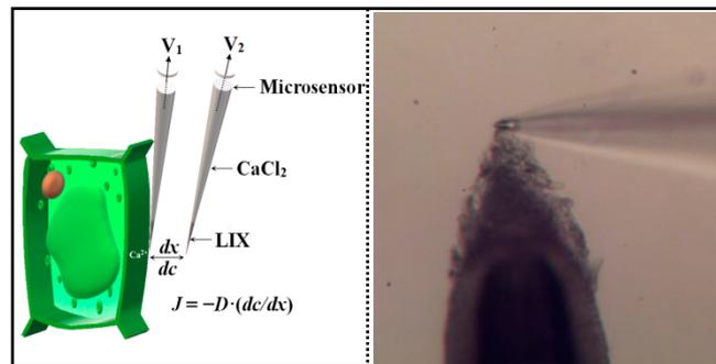
**Figure 2.** Schematic diagram and measured photo of  $\text{Ca}^{2+}$  flux analysis by non-invasive micro-tests. The diagram is to demonstrate the principles behind NMT testing and is not to scale. The tip diameter of the microsensor is about  $5\ \mu\text{m}$ .
