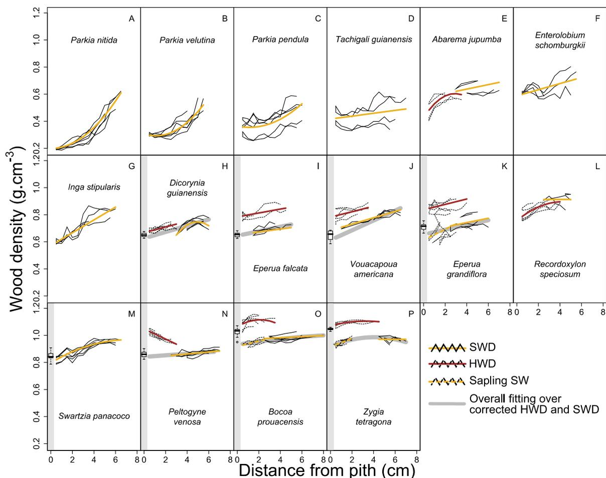
**Figure 4.** Modeling of radial patterns in wood density according to radial distance for heartwood free species (A, B, C, D, F, G, and M) and for species with heartwood (E, H, I, J, K, L, N, O, and P). Red and yellow solid lines represent the fixed effect of the best fit for heartwood and sapwood respectively. Yellow dotted lines represent the fixed effect of the best fit for the sapwood of the
