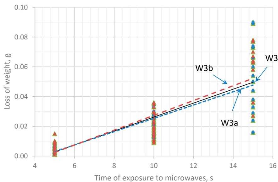
**Figure 5.** Dependence between loss of weight and time of exposure to microwaves in the third measurement mode (W3, W3a, W3b).
