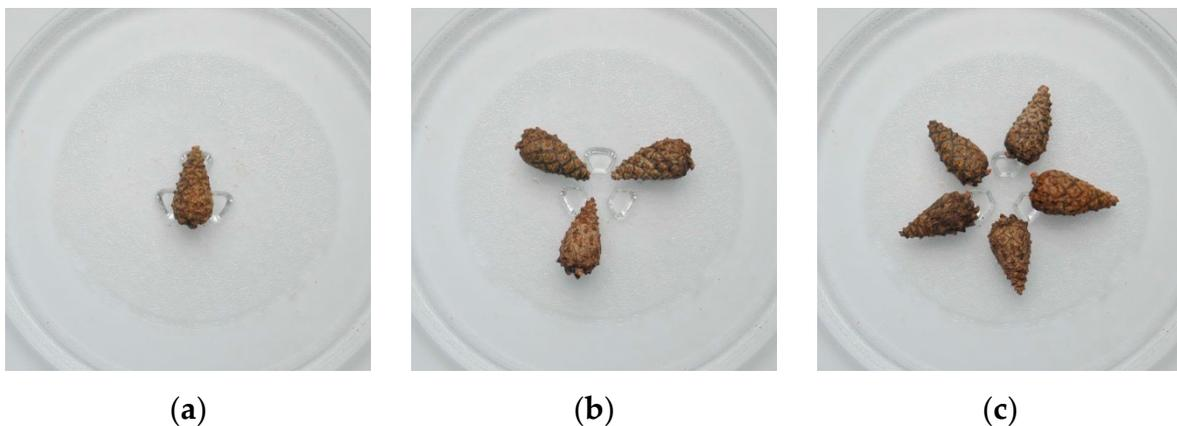
**Figure 2.** Cone arrangement on the turntable: (a) single cone (W1); (b) three cones with apexes pointing towards the centre (W2a); (c) five cones with apexes pointing towards the edge (W3b).
