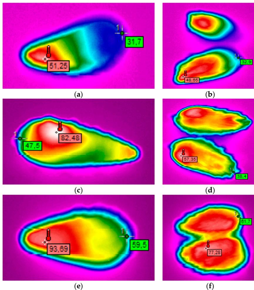
**Figure 7.** Thermal images of cone heating: (a) whole cone with the apex pointing outwards, heated for 5 s; (b) cone halves with the apex pointing outwards, heated for 5 s; (c) whole cone with the apex pointing centrewise, heated for 10 s; (d) cone halves with the apex pointing centrewise, heated for 10 s; (e) whole cone with the apex pointing outwards, heated for 15 s; and (f) cone halves with the apex pointing outwards, heated for 15 s.
