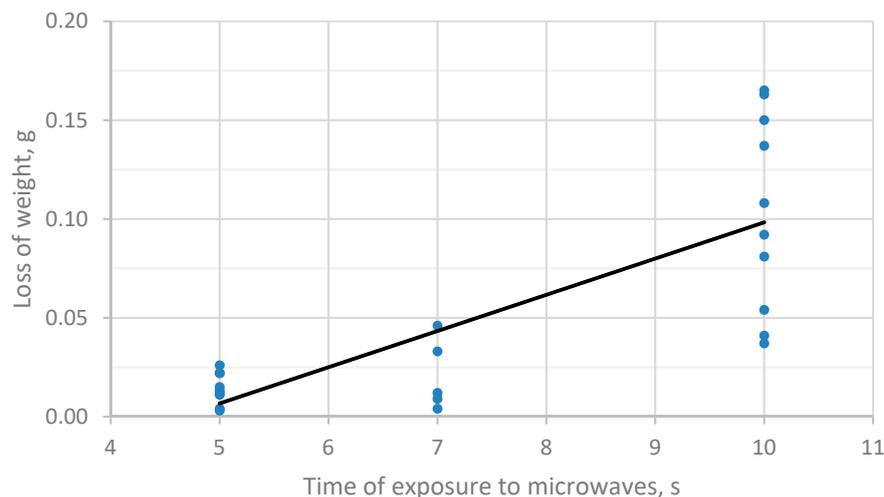
**Figure 3.** Dependence between loss of weight and time of exposure to microwaves in the first measurement mode (W1).
