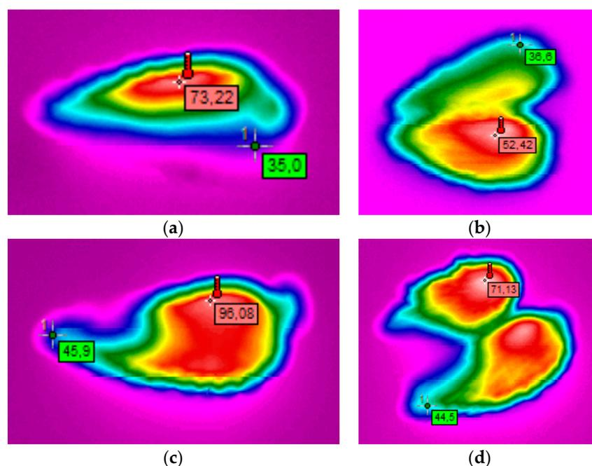
**Figure 6.** Thermal images of cone heating in the study mode W1: (a) whole cone, 7 s; (b) cone halves, 7 s; (c) whole cone, 10 s; and (d) cone halves, 10 s.
