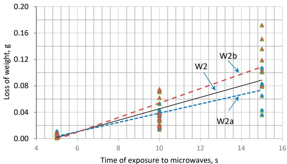
**Figure 4.** Dependence between loss of weight and time of exposure to microwaves in the second measurement mode (W2, W2a, W2b).
