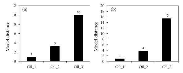
**Figure 4.** Model distance plot for the three oils on the wood samples: (a) *Cryptomeria japonica;* (b) *Chamaecyparis obtusa.*
