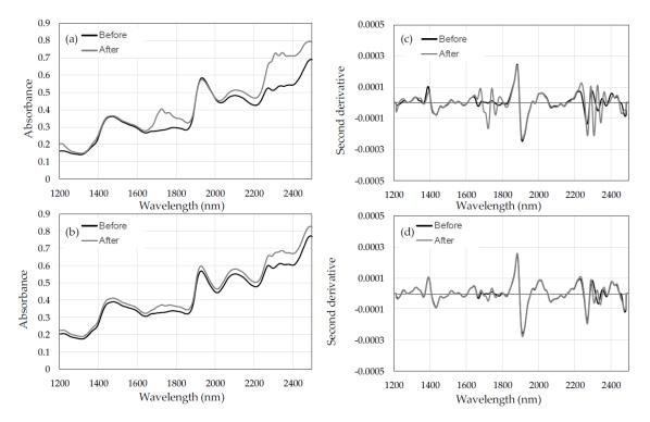
**Figure 2.** NIR spectra of *Cryptomeria japonica* (**a**,**c**) and *Chamaecyparis obtusa* (**b**,**d**) flat grain samples. (**a**,**b**) are raw spectra, and (**c**,**d**) are pre-processed spectra. Black lines indicate the spectra collected before applying Oil\_1, and the gray lines indicate those obtained after applying Oil\_1 to the surfaces of the wood samples.
