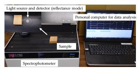
Figure 1. Outline of measurement device.
