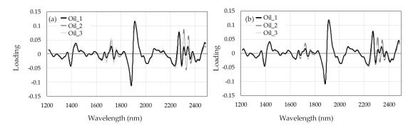
Figure 3. PC1 loading plots for oil-treated (a) Cryptomeria japonica and (b) Chamaecyparis obtusa.
