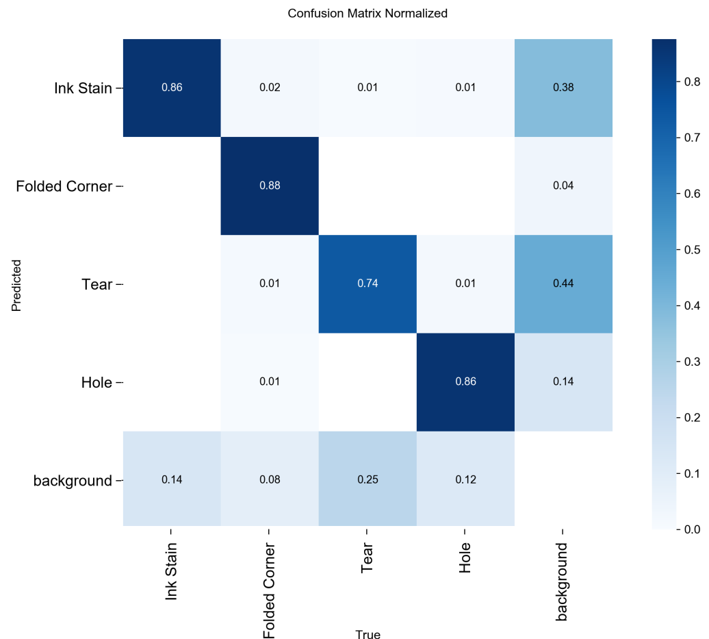
Figure 7. Normalized confusion matrix of LME-YOLO on the book defect test set.
