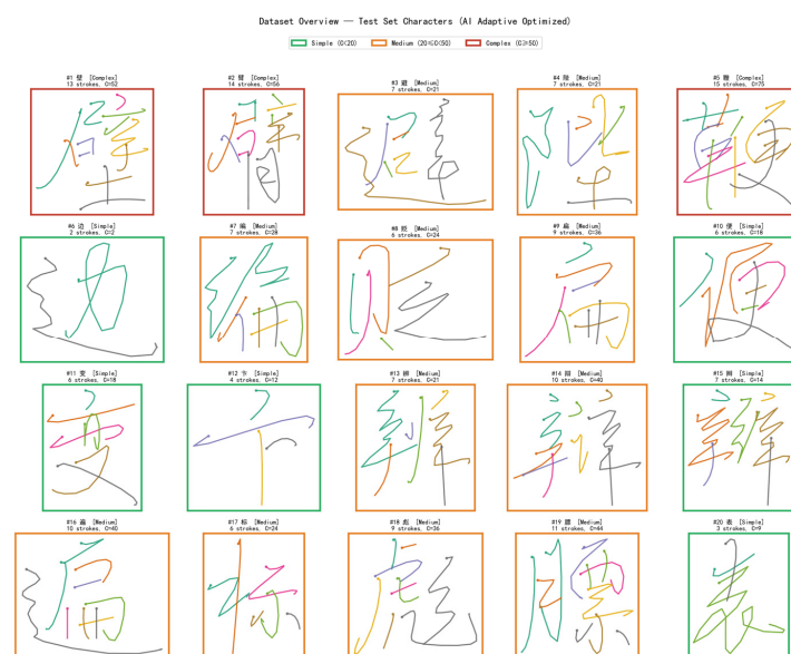
Figure 20. AI Adaptive optimized stroke trajectories for the first 20 holdout test characters. Each character is rendered with complexity-aware parameters ( \sigma and interpolation factor adapted per tier). Border color indicates complexity tier (green: Simple, orange: Medium, red: Complex). Compared with the original trajectories in Figure 13b, the optimized versions show smoother curves with preserved structural fidelity.
