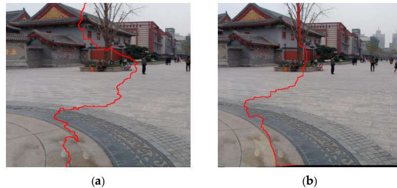
Figure 3. Comparison of the optimal stitching seams. (a) Seam generated by conventional seam-cutting; (b) Seam generated by the proposed quality-aware seam-cutting.
