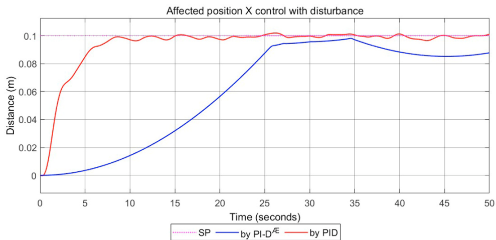
Figure 28. System with disturbance and PID position control affected by equilibrium controllers.
