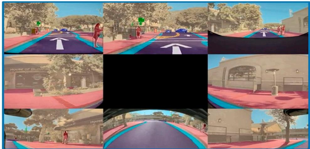
**Figure 13.** Autonomous driving using panoptic segmentation (Andrej Karpathy) [45].
