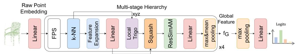
**Figure 2.** Overall structure of Point-SimP. Different colors represent different module types in the network.
