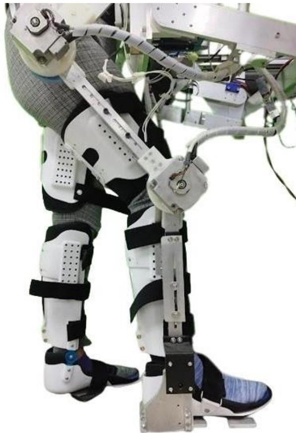
**Figure 7.** Developed prototype of a rehabilitation exoskeleton to assist the ankle and knee in ACL injury exercises.
