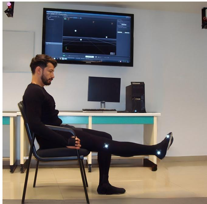
**Figure 4.** Motion capture system to obtain the desired trajectory or adequate rehabilitation routine, through a vision system with 12 cameras.
