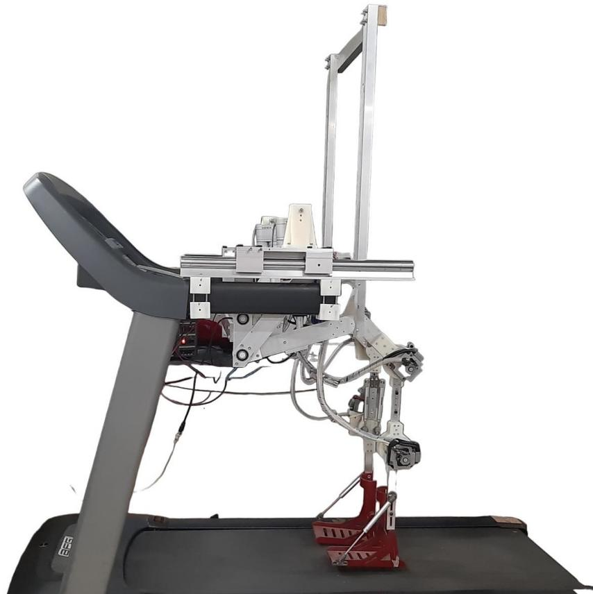
**Figure 1.** Exoskeleton for gait rehabilitation to assist in the task of standing–sitting the patient and the hip and knee movements [9].
