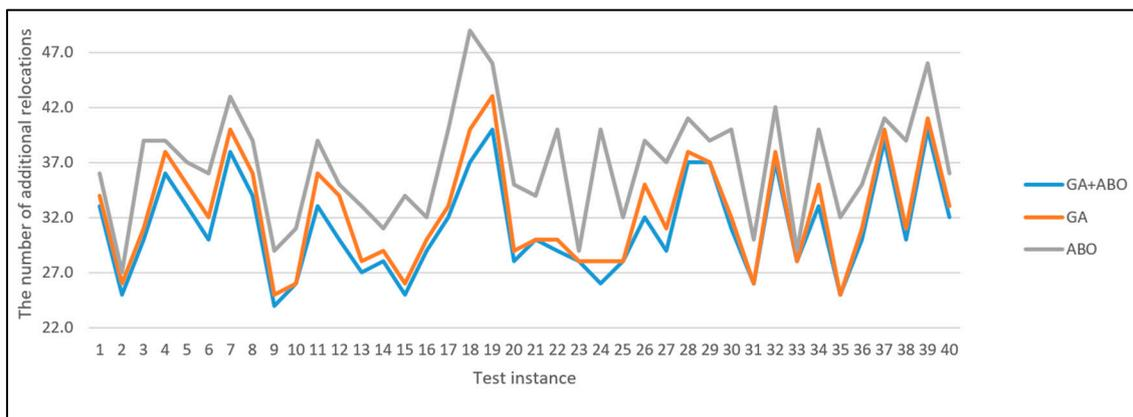
**Figure 6.** A comparison of the optimization results (the number of additional relocations) of the GA+ABO, GA, and ABO for all 40 instances of the CRP test set with size of  $6 \times 7$  for tests with combination values of *ITN* and *PS*  $500 \times 1000$ .
