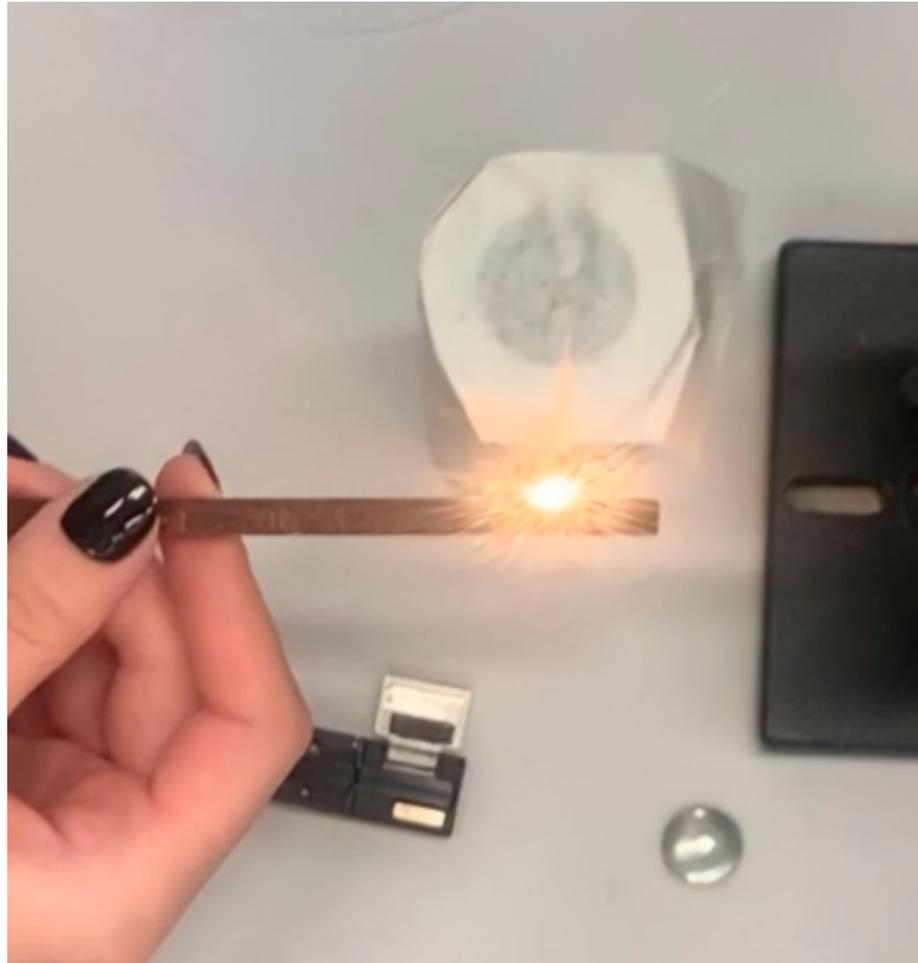
**Figure 2.** The moment of plasma spark initiation in the fiber.
