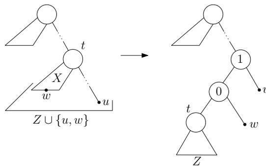
**Figure 7.** (left) The  $P_4$ -sparse tree  $T_{OPT}$  in which the leaves for  $u, w$  do not have the same parent node and have node  $t$  as their least common ancestor; (right) The  $P_4$ -sparse tree  $T_R$  obtained by using Formation 2 just above node  $t$  which results in no more fill edges than those in  $G_{OPT}$ .
