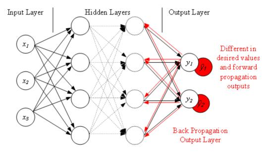
Figure 1. Illustration diagram shows how a Back Propagation Neural Network works.
