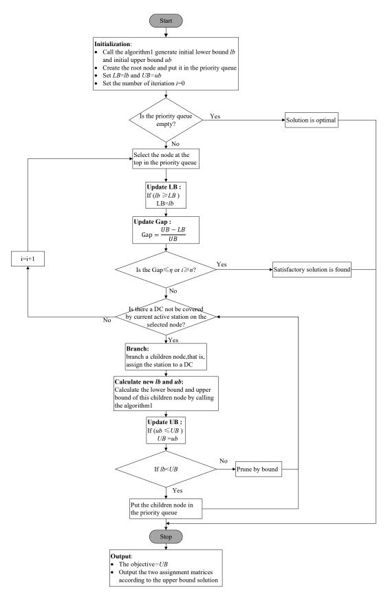
Figure 15. Flowchart of the customized branch-and-bound algorithm.
