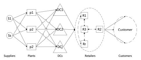
Figure 1. A five-echelon supply chain network with lateral-transshipments in retailers [6].
