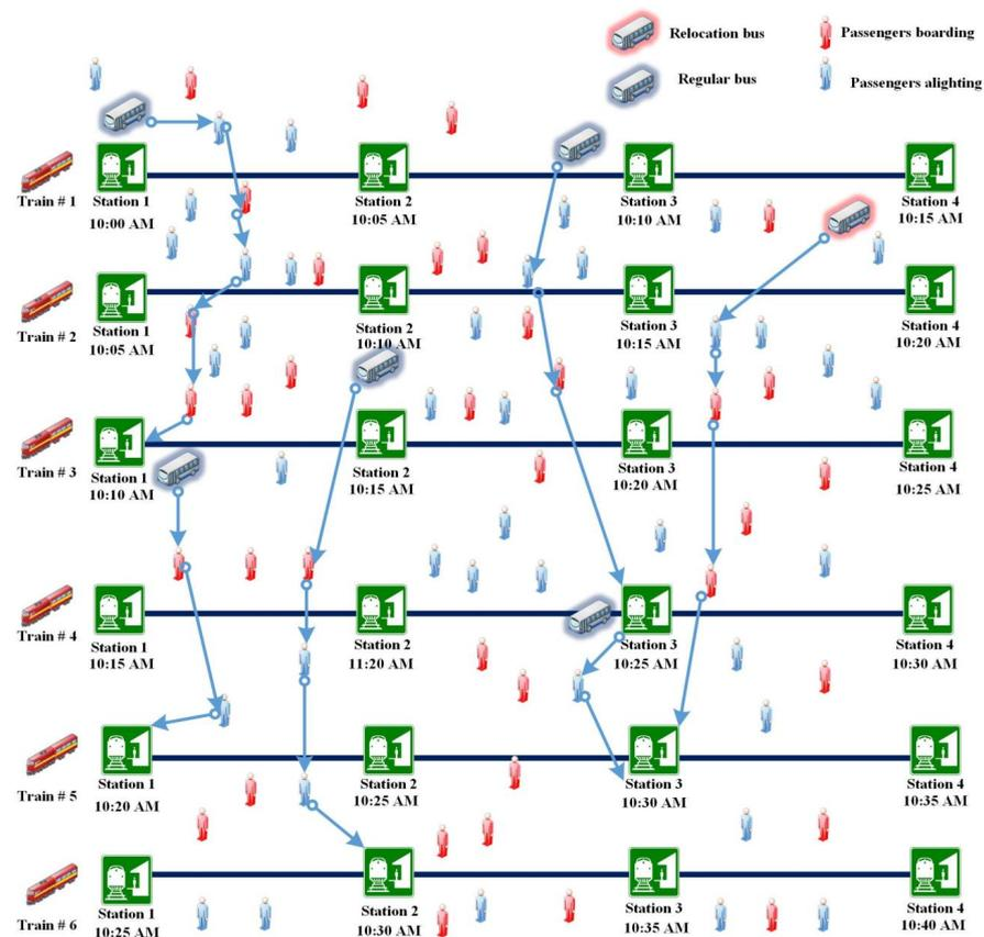
Figure 1. Conceptual operation of the proposed demand-responsive feeder transit service.
