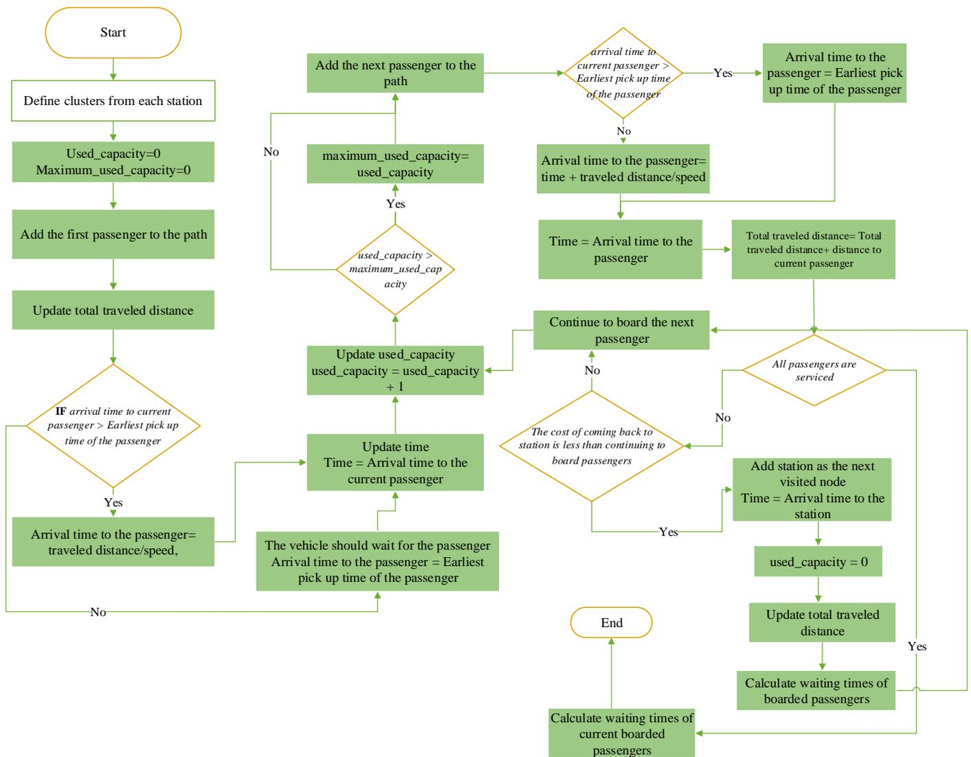
Figure 3. The path creator algorithm.
