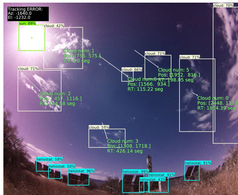
Figure 2. Cloud detection results. White, blue, and green boxes to show cloud, heliostat, and sun detection, respectively.
