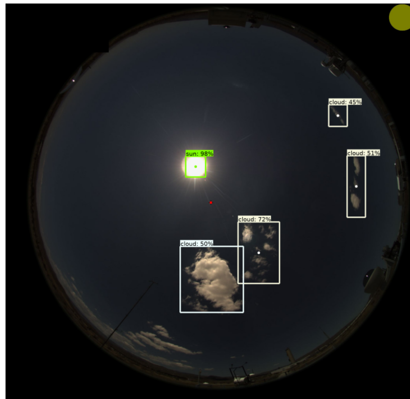
Figure 9. Object detection results from a Mobotix Q25 camera image.
