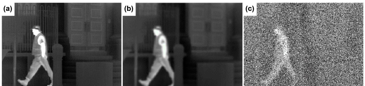
**Figure 2.** The passerby image with different degrees of degradation. (a) The original image, (b) the  $7 \times 7$  Gaussian blur, and (c) the  $7 \times 7$  Gaussian blur + 30% salt-and-pepper noise.
