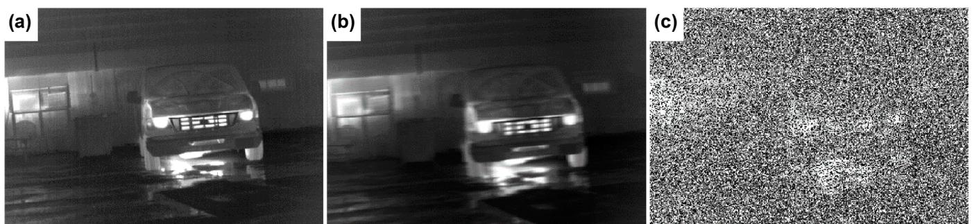
**Figure 6.** The truck image with different degrees of degradation. (a) The original image, (b) the  $7 \times 7$  motion blur, and (c) the  $7 \times 7$  motion blur + 50% salt-and-pepper noise.
