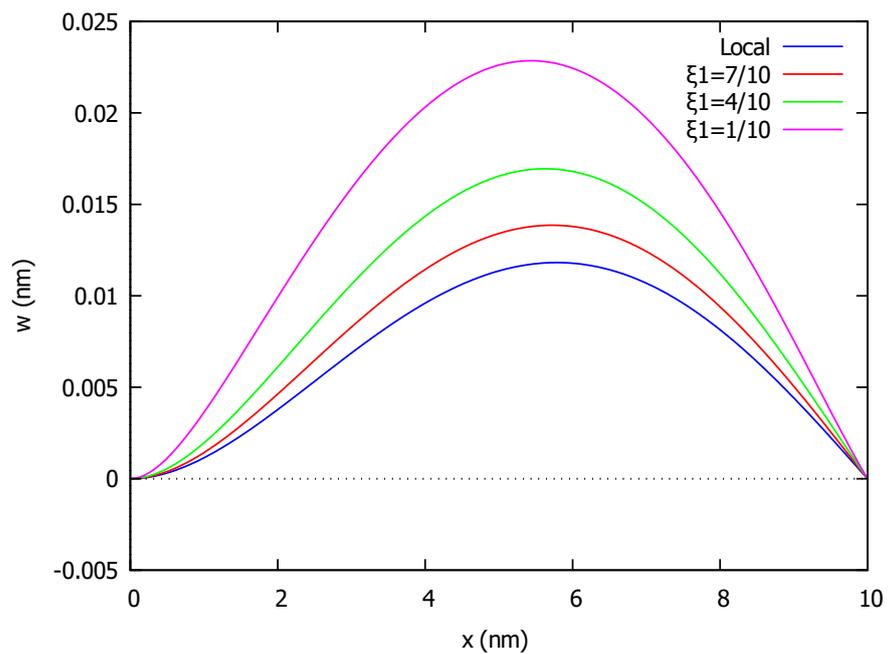
Figure 5. Deflection of clamped pinned beam (CP) under uniform load and various values of  $\zeta_1$ .
