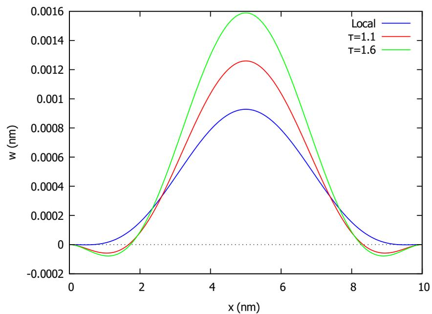
Figure 9. Deflection of clamped beam (CP) under variable load and different values of  $\tau$ .
