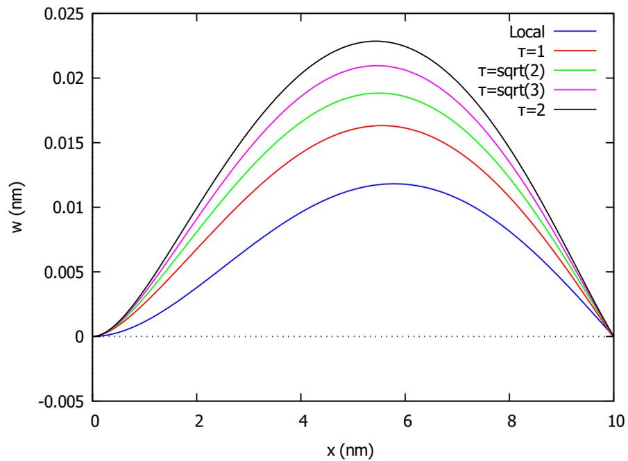
Figure 4. Deflection of clamped pinned beam (CP) under uniform load and several values of  $\tau$ .
