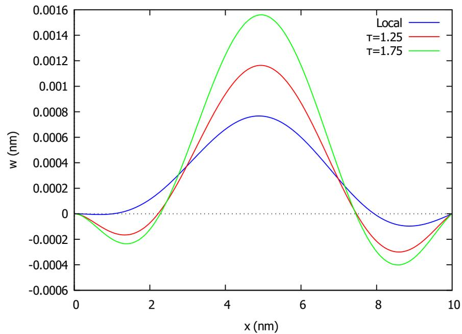
Figure 6. Deflection of clamped pinned beam (CP) under variable load and different values of  $\tau$ .
