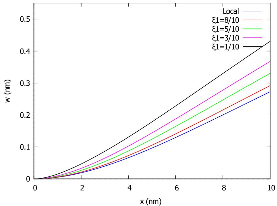
Figure 2. Deflection of cantilever beam (CF) under uniform load and several values of  $\zeta_1$ .
