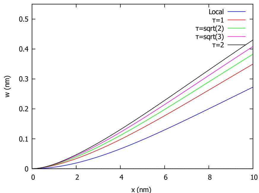
**Figure 1.** Deflection of cantilever beam (CF) under uniform load and various values of  $\tau$ .
