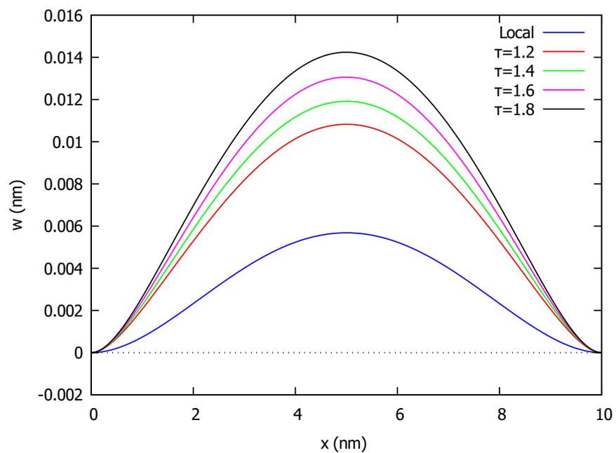
Figure 7. Deflection of clamped beam (CP) under uniform load and several values of  $\tau$ .
