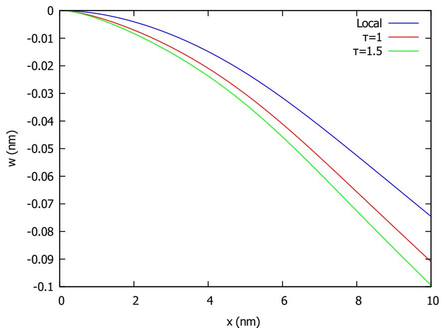
Figure 3. Deflection of cantilever beam (CF) under variable load and different values of  $\tau$ .
