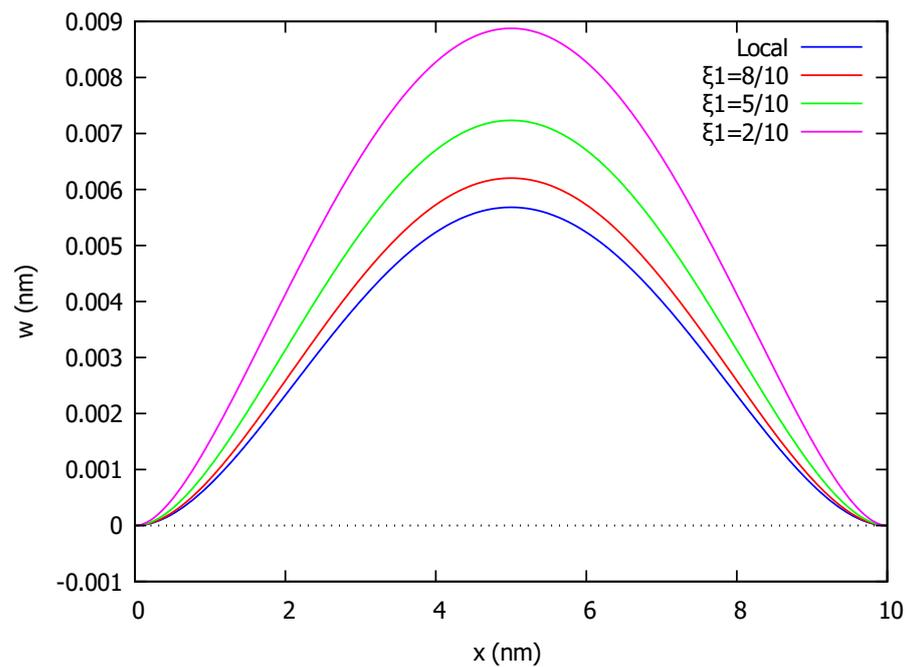
Figure 8. Deflection of clamped beam (CP) under uniform load and various values of  $\zeta_1$ .
