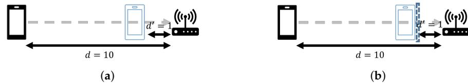
Figure 6. Schematic of the RVPV environment: (a) LOS condition; (b) NLOS condition.
