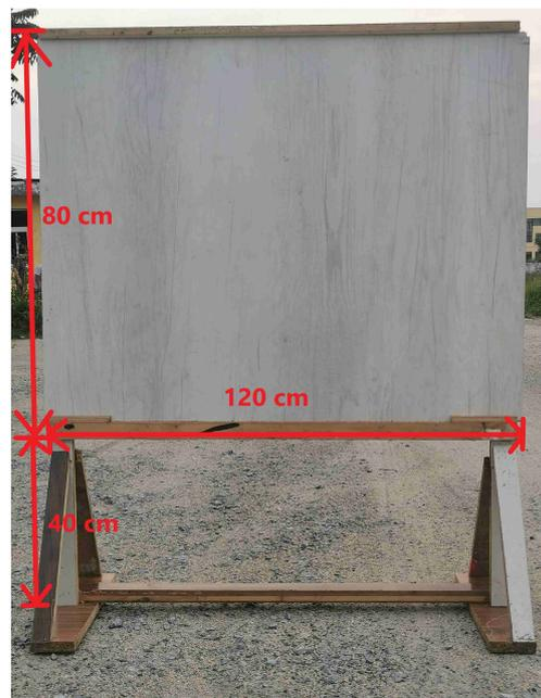
Figure 2. Specification of the frame and the blocker (metal in this figure).
