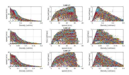
Figure 5. Speed, density, and flow plot of links in the network.
