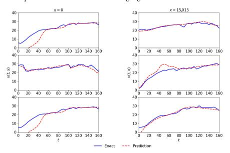
**Figure 12.** Actual and predicted speed at two intersections i.e., at x = 0 and x = 15,015 m, respectively given by the first and second columns. The first, second, and third rows respectively represent the network's links L1, L2, and L3.
