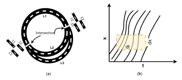
**Figure 3.** (a) Traffic network with three links and two intersection points; (b) the trajectories of the vehicles and a discrete area to estimate the traffic states.
