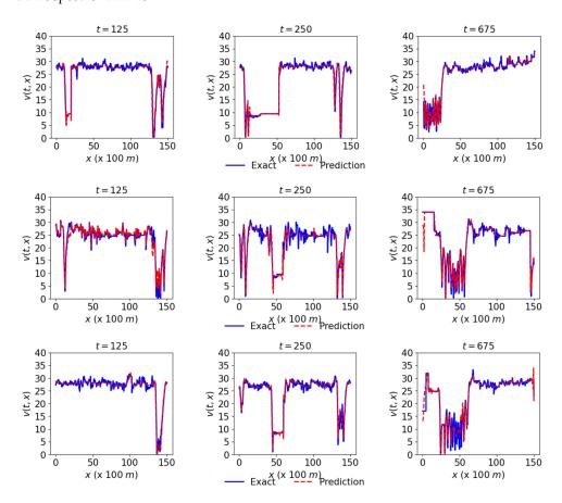
**Figure 7.** Actual and predicted speed at three different times 125, 250, and 675 respectively given by the first, second, and third columns. The first, second, and third rows respectively represent the network's links L1, L2, and L3.
