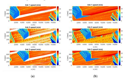
**Figure 4.** (a) Speed contour plot showing cells where no vehicle detected; (b) speed contour where missing cells filled with the speed of neighboring cells.
