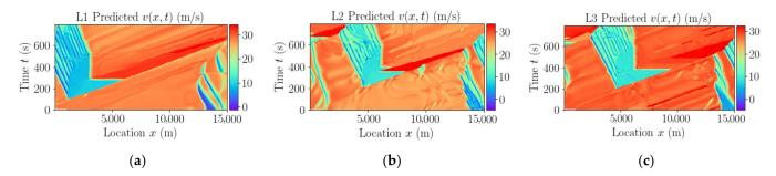
**Figure 6.** (a) Predicted traffic speed of Link L1, (b) predicted traffic speed of Link L2; (c) predicted traffic speed of Link L3.
