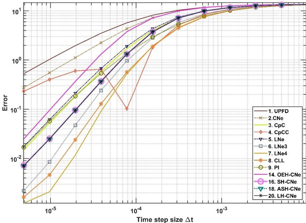
Figure 15. The maximum errors as a function of the time step size  $\Delta t$  for the slowly converging methods in the case of Experiment 6, where the diffusion constant strongly depends on the time.
