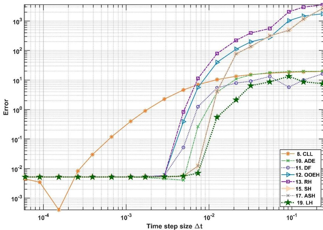
Figure 12. The errors as a function of the time step size for the quickly converging methods, as well as the CLL method, in the case of Experiment 5.
