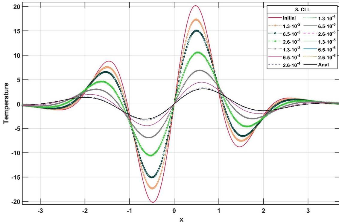
**Figure 5.** The numerically calculated temperatures  $u$  for the three-stage CLL method as a function of the space variable  $x$  for different time step sizes in Experiment 1. The red and the black solid lines are for the initial and the analytically calculated temperatures, respectively.
