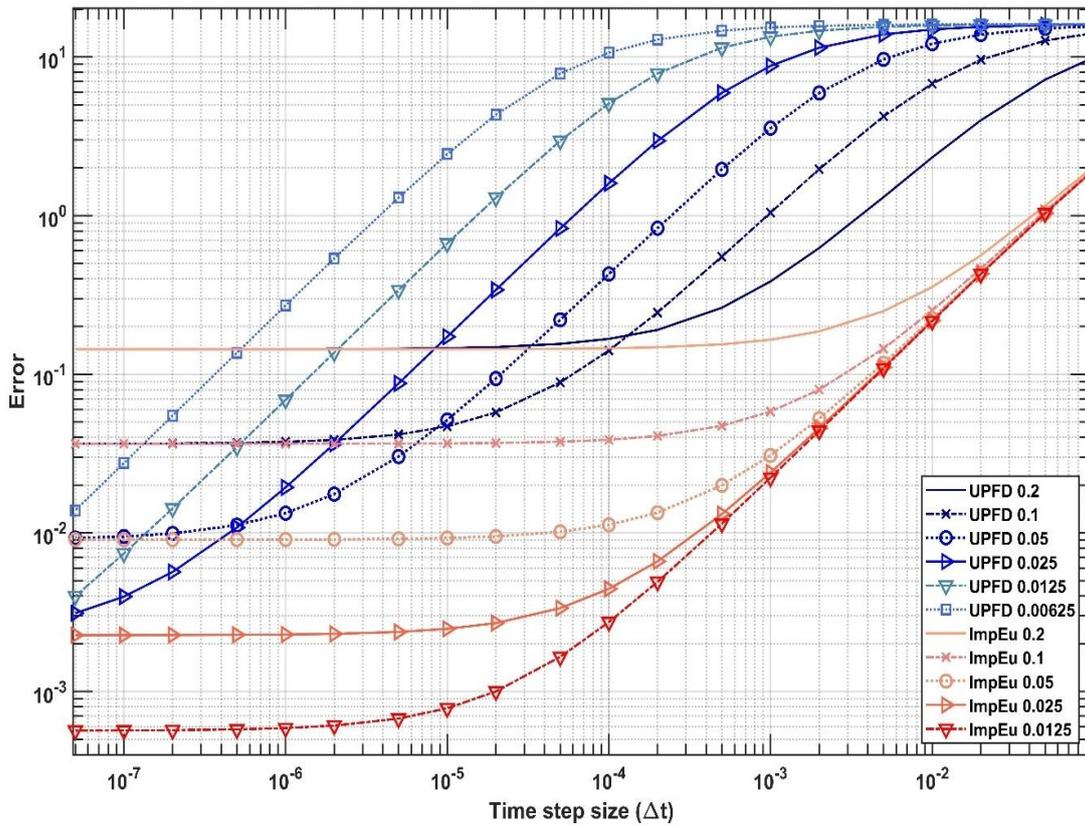
Figure 8. Errors as a function of the time step size for the UPFD and the implicit Euler (ImpEu) methods with different space step sizes in Experiment 3.  $\Delta x$  changes from 0.2 to 0.00625 and to 0.0125 for the UPFD and the implicit method, respectively.
