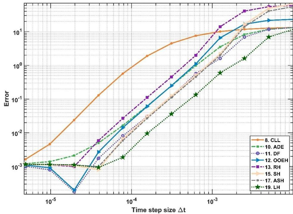
Figure 16. The maximum errors as a function of the time step size  $\Delta t$  for the fast convergent numerical schemes in the case of Experiment 6.
