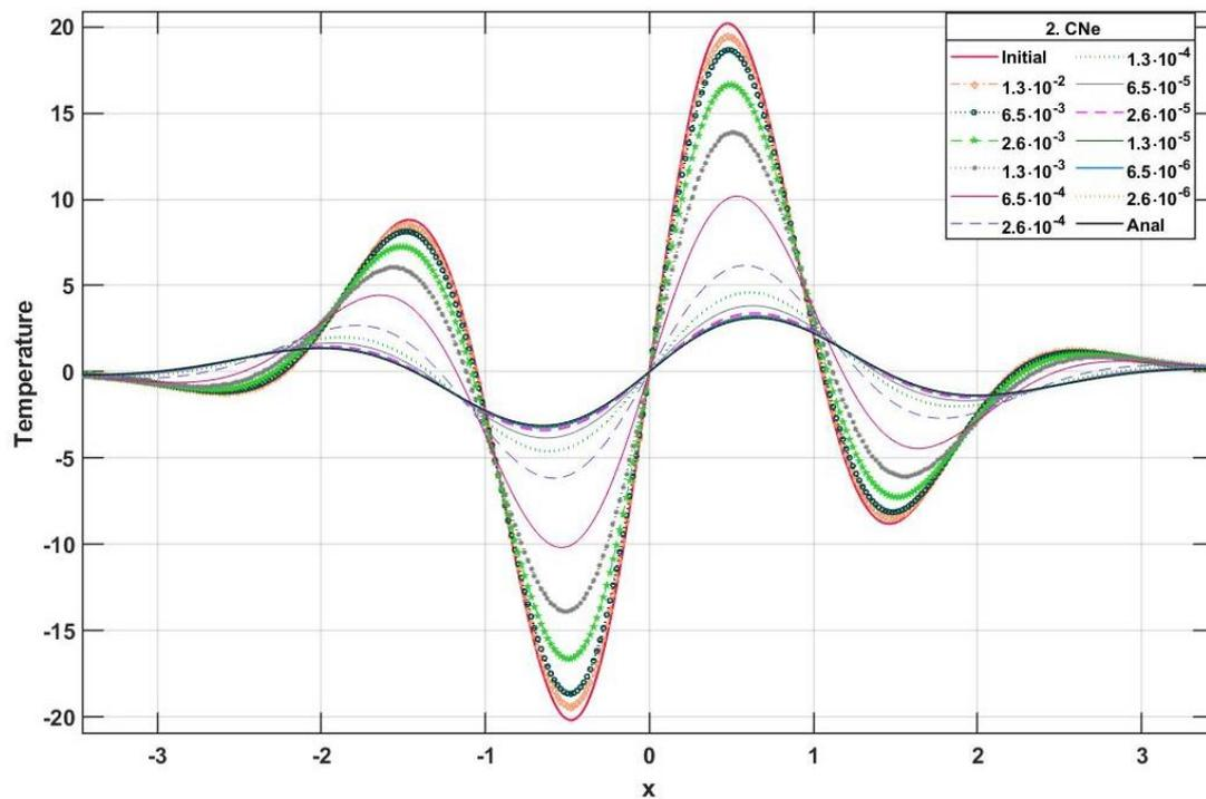
**Figure 4.** The numerically calculated temperatures  $u$  for the three-stage CNe method as a function of the space variable  $x$  for different time step sizes in Experiment 1. The red and the black solid lines are for the initial and the analytically calculated temperatures, respectively.
