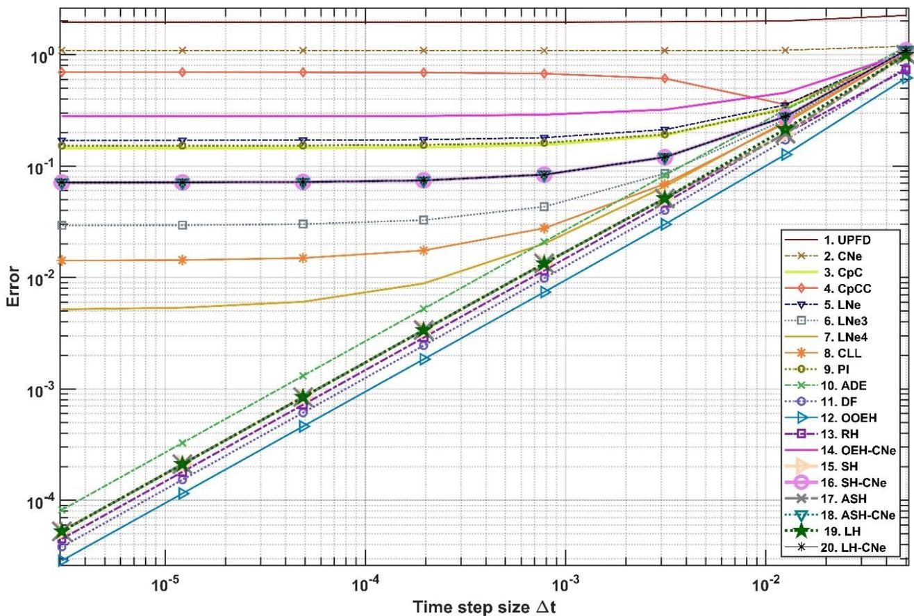
Figure 10. The maximum errors as a function of the time step size in Experiment 4 for a constant  $r = \alpha \Delta t / \Delta x^2$ . This means that the space step size also decreases from the right to the left side of the figure.
