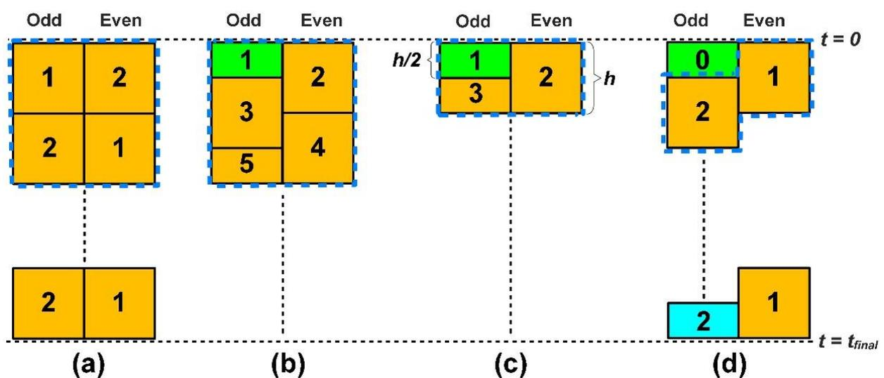
**Figure 1.** Space-time structure of the hopscotch-type algorithms. (a) Original odd–even hopscotch (OOEH), (b) shifted-hopscotch (SH), (c) asymmetric hopscotch (ASH), (d) leapfrog-hopscotch (LH).
