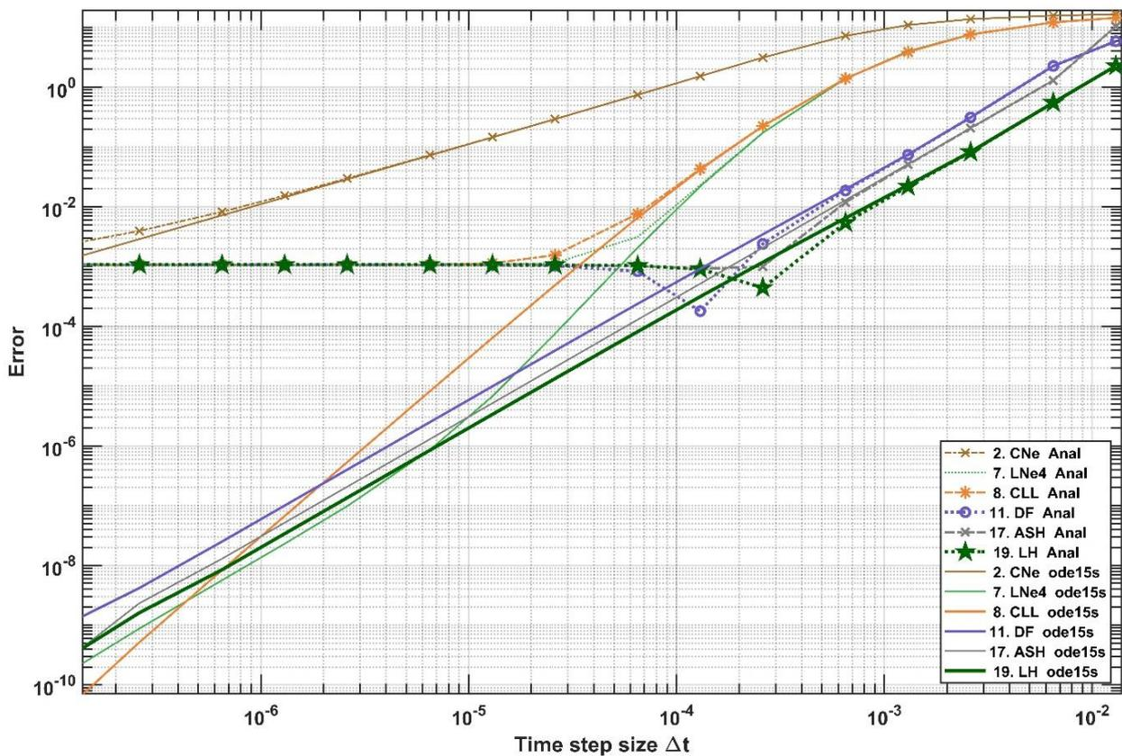
**Figure 7.** The errors as a function of the time step size for six methods in Experiment 2 when not only the analytical but a numerical reference solution was used to calculate the errors.
