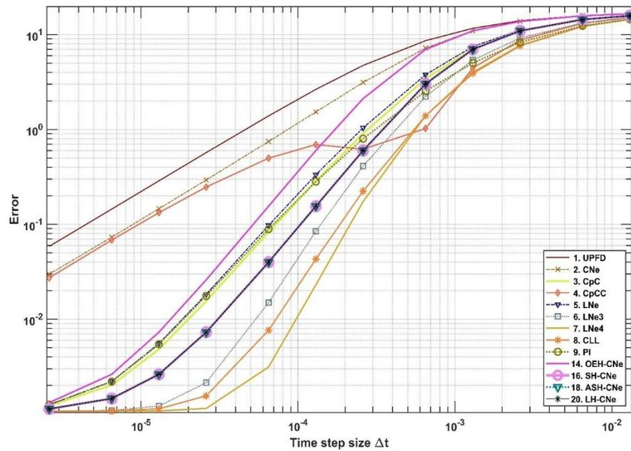
Figure 2. Errors as a function of the time step size for the slowly converging methods.
