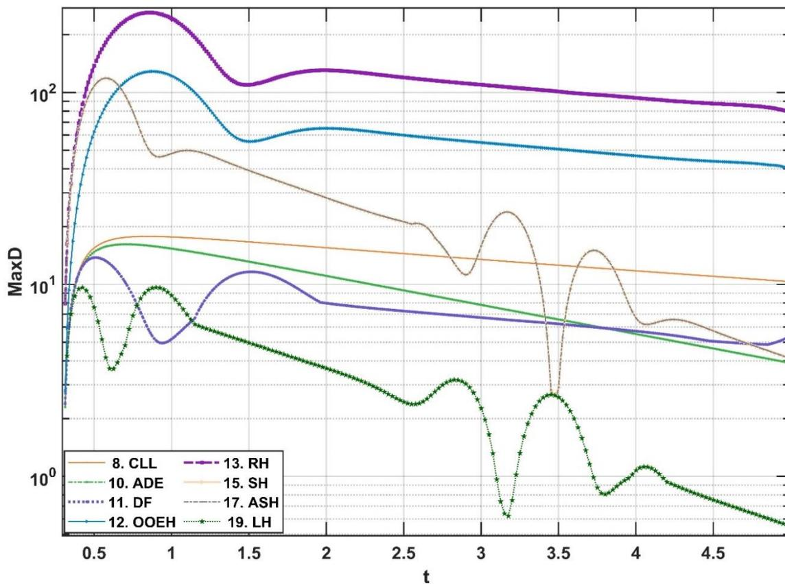
Figure 14. The evolution of the maximum errors as a function of the physical time  $t$  in the case of fast converging methods in Experiment 5. The used time step size is rather large:  $\Delta t = 1.25 \cdot 10^{-2}$ .
