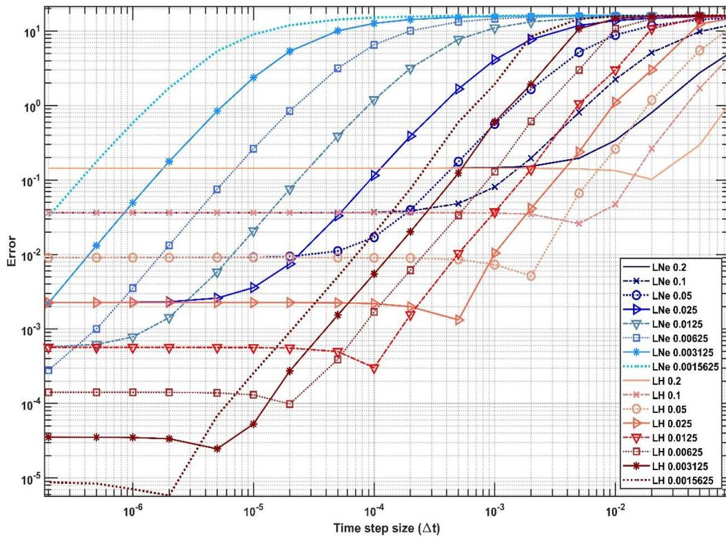
Figure 9. Errors as a function of the time step size for the LNe and the LH methods with different space step sizes in Experiment 3.
