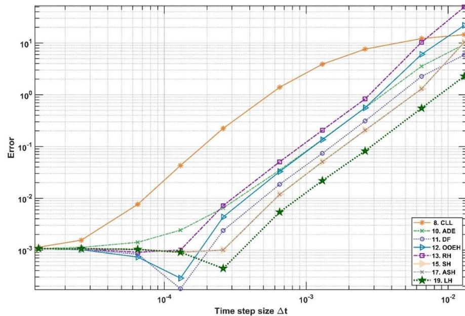
Figure 3. The errors as a function of the time step size for the quickly converging methods, as well as the CLL method in the case of Experiment 1. The error curves reach the residual error  $\tau_0$  on the left side of the figure.
