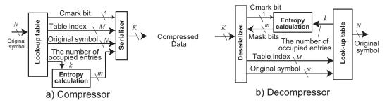
Figure 1. Organization of Compressor/Decompressor in ASE coding.
