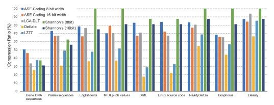
**Figure 7.** Comparisons of compression ratios among ASE coding (8/16 bit symbol input) and the conventional methods.
