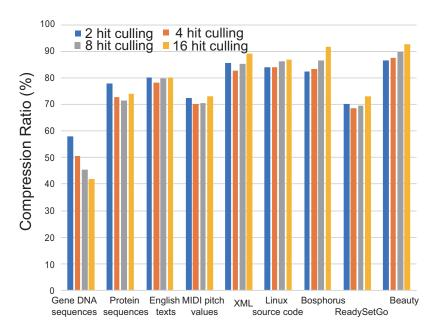
**Figure 9.** Comparisons of compression ratios of ASE coding with varying the number of hit counting of entropy culling.
