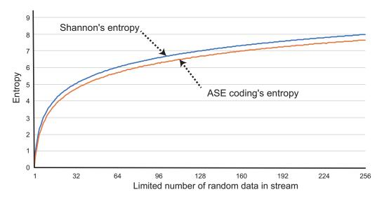
Figure 5. Entropy comparison between Shannon's and ASE coding's.
