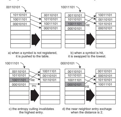
Figure 4. Look-up table operations in Adaptive Stream-based Entropy (ASE) coding.
