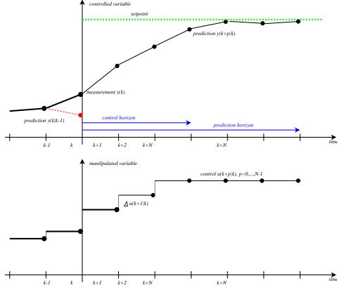
Figure 2. Receding horizon predictive control principle.
