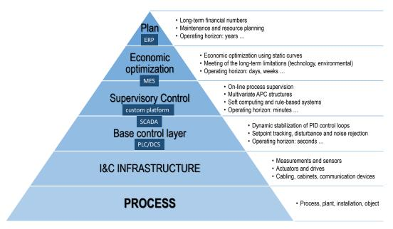
Figure 1. The hierarchical layout of a control system. APC, Advanced Process Control.
