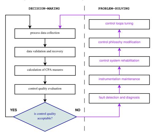
Figure 3. CPA industrial utilization process.
