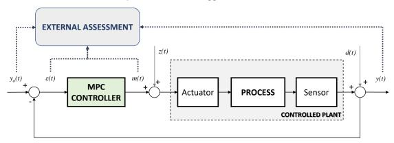
Figure 6. MPC external approach to the CPA.
