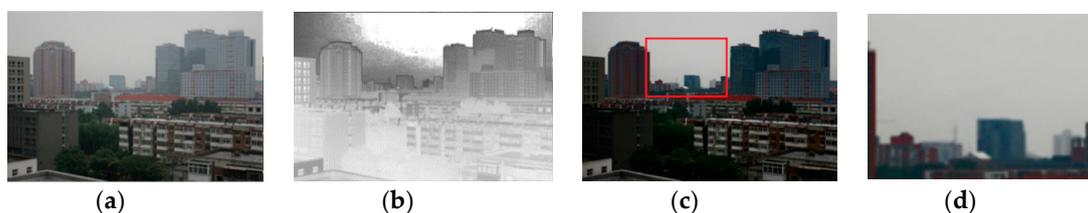
Figure 6. (a) hazy image. (b) Transmission map. (c) Restored image with (b). (d) Magnification of rectangle (c).
