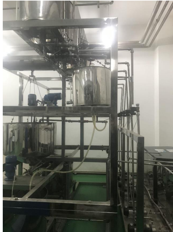
Figure 6. GM&D-A type particleboard glue mixing and dosing device.
