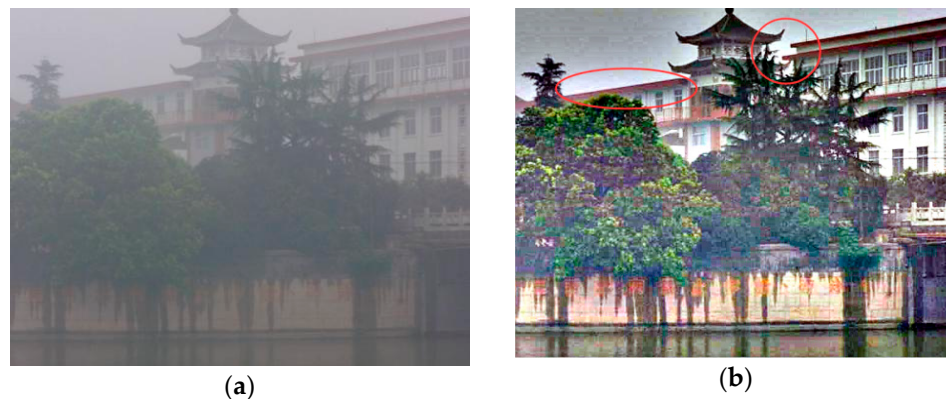
Figure 2. Illustration of the limitations of the single-scale Retinex (SSR) algorithm. (a) Input image. (b) Result of SSR enhancement. The "halo" effect observed in areas with significant changes in local color is marked in red.
