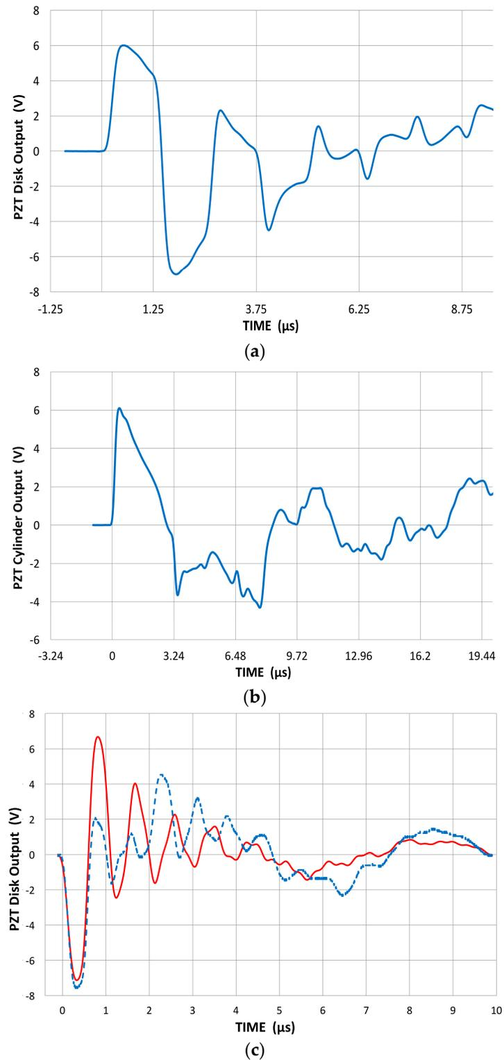
**Figure 12.** Output signals from PZT disks and cylinder, coupled to V104 reference transmitter. (a) Output signals from 400 kHz PZT disk; (b) Output signals from 160 kHz PZT cylinder; (c) 1 MHz disk with brass backing (blue, dash) and without backing (red).
