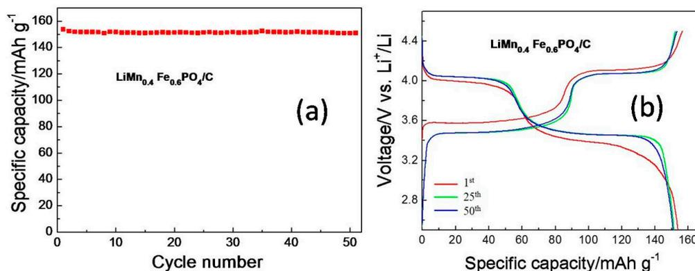
**Figure S2.** (a) Cycling performance at 0.1 C ( $1\text{ C} = 170\text{ mA}\cdot\text{g}^{-1}$ ) and (b) voltage profile of  $\text{LiMn}_{0.4}\text{Fe}_{0.6}\text{PO}_4/\text{C}$  composite material prepared by  $\text{LiMnPO}_4$  nano-plates and  $\text{LiFePO}_4$  nano-plates.
