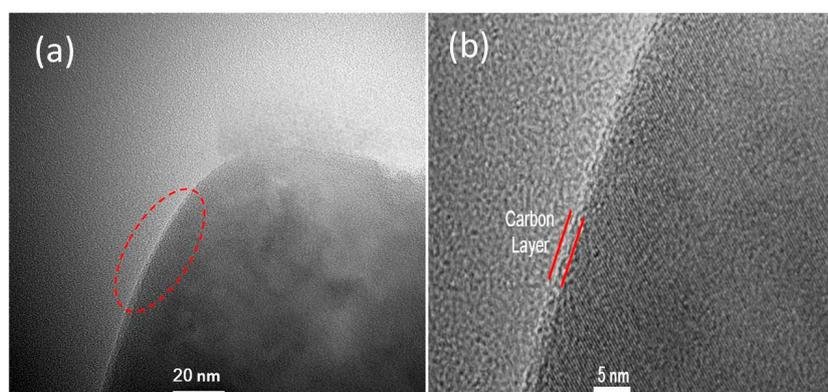
**Figure S1.** (a) TEM and (b) magnified TEM images of  $\text{LiMn}_{0.4}\text{Fe}_{0.6}\text{PO}_4/\text{C}$  composite materials.
