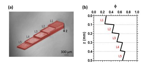
**Figure 7.** (a) Example of a UV cured sample made of coloured diacrylate, printed by setting 100  $\mu$ m as single layer thickness; (b) profile of the step-gradient conversion  $\phi$  along the sample depth *z*, modelled using the optical attenuation coefficient of the system ( $\mu = 1.54 \text{ mm}^{-1}$ ).
