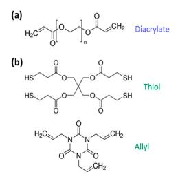
**Figure 2.** Chemical structure of model monomers used in this work: poly(ethylene glycol) diacrylate (diacrylate) (**a**); and thiol-allyl system (**b**), formed by 1,3,5-triallyl-1,3,5-triazine-2,4,6(1H,3H,5H)-trione and pentaerythritol tetrakis(3-mercaptopropionate) (these two monomers were mixed assuring an equimolar amount of allyl and thiol reactive groups).
