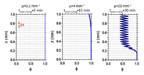
**Figure 8.** Conversion  $\phi$  profiles along the sample depth *z* for 3D printed objects after post-curing. The layer thickness during the printing process ( $\Delta z$ ) is set as 50 µm. Profiles are modeled imposing  $\mu = 0.2 \text{ mm}^{-1}$ ,  $\mu = 4 \text{ mm}^{-1}$  and  $\mu = 20 \text{ mm}^{-1}$ ,  $I = 3 \text{ W} \cdot \text{m}^{-2}$ , and the post-curing time as 5 min, 15 min and 30 min, respectively.
