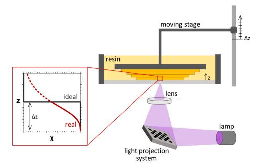
**Figure 1.** Schematic of a bottom-up 3D printer based on photopolymerisation. Each processed layer, with a thickness equal to  $\Delta z$ , is characterized by a non-constant monomer-to-polymer conversion  $\chi$ , which shows a sigmoidal profile (**red**), and differs from the ideal square profile (**black**).
