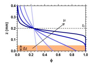
**Figure 5.** Conversion  $\phi$  profiles along the sample depth *z* for increasing attenuation coefficient  $\mu$ . The position of the photopolymerising front  $z_f$  is fixed equal to 200 µm, and the printing layer thickness  $\Delta z$  is set as 50 µm.
