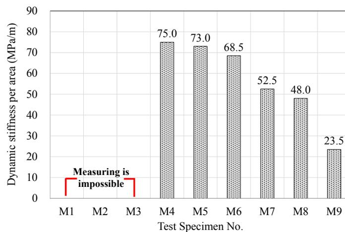
**Figure 9.** Variations of dynamic stiffness according to mixing conditions.
