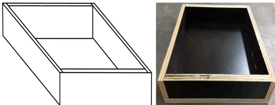
**Figure 1.** A mold for specimen of a place-type resilient material.
