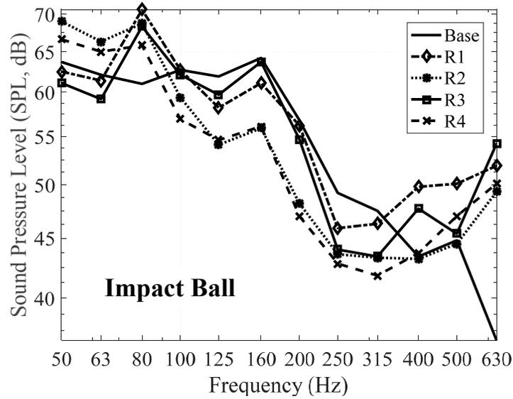
Figure 15. Floor impact sound level with the proposed materials in 1/3 Octave bands—Impact ball.
