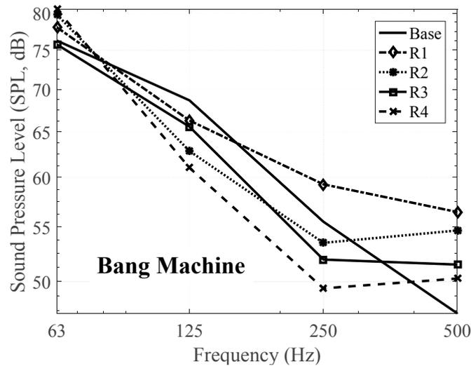
Figure 18. Floor impact sound level with the proposed materials in 1/1 Octave bands—Bang machine.
