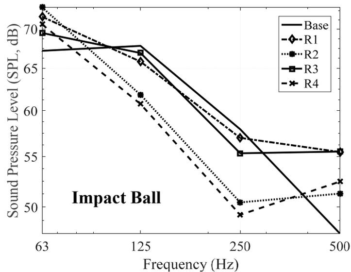
Figure 16. Floor impact sound level with the proposed materials in 1/1 Octave bands—Impact ball.
