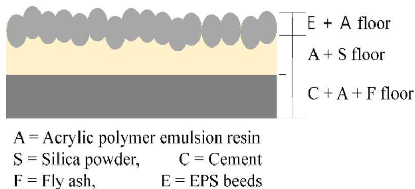
**Figure 2.** Schematic diagram of the place-type resilient material.
