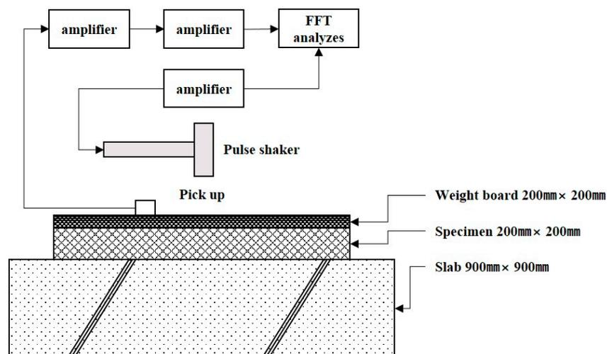
Figure 4. Test method for dynamic stiffness by pulse shaker.
