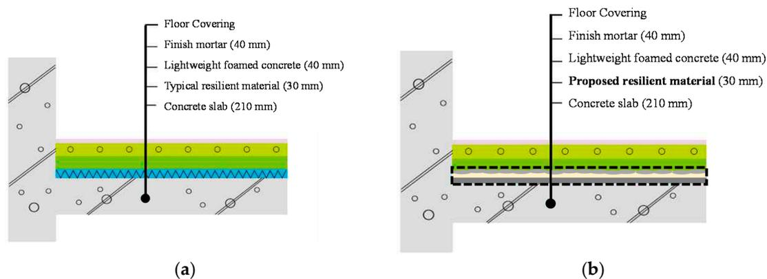
**Figure 11.** Schematic overview of floor system with resilient materials installation: (a) typical floor system; and (b) proposed floor system.
