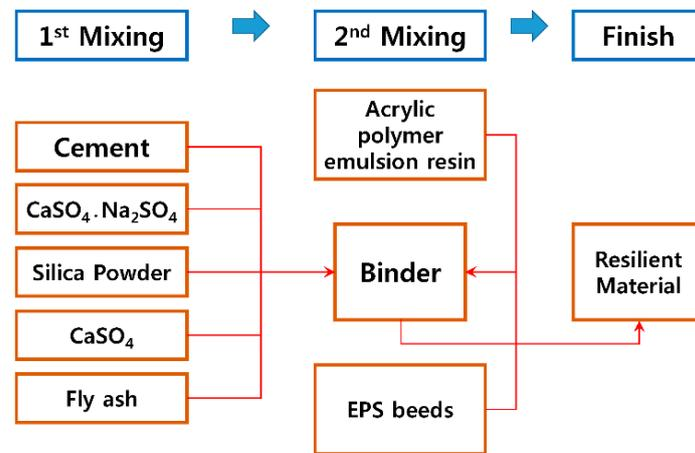
Figure 3. Experiment process of the place-type resilient material.
