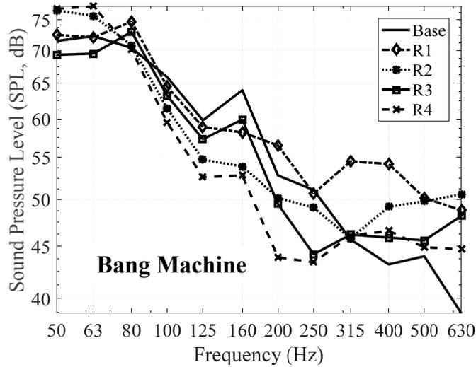
Figure 17. Floor impact sound level with the proposed materials in 1/3 Octave bands—Bang machine.
