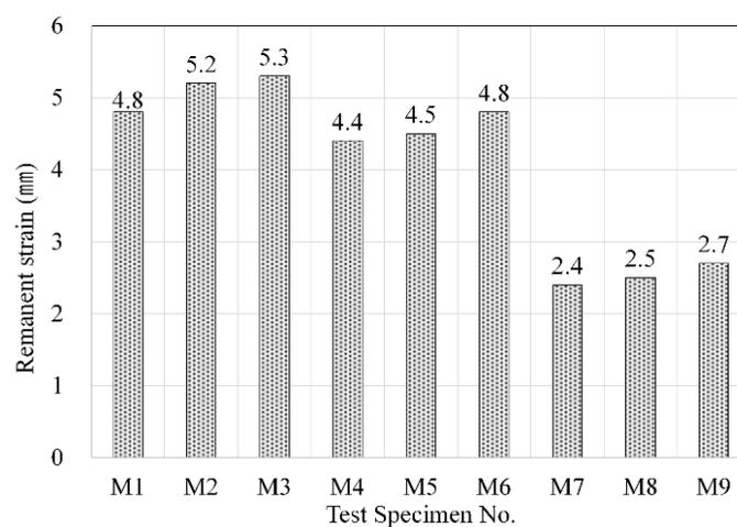
Figure 10. Variations of remanent strain according to mixing conditions.
