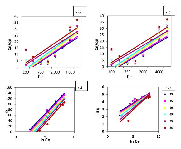
**Figure 15.** Equilibrium isotherm models for the copper sorption process at different solution temperatures (amount of MANSG = 0.25 g; agitation speed = 200 rpm; solution volume = 25 mL; pH = 7): (a) Langmuir isotherm model; (b) Freundlich isotherm model; (c) Temkin isotherm model; (d) Elovich isotherm model.
