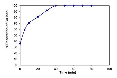
Figure 14. Desorption kinetics of copper ions from MANSG using 0.02 N EDTA.
