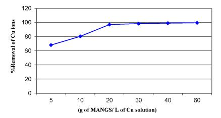
**Figure 10.** Effect of the MANSG dose on the copper sorption process (solution concentration of ion = 1000 ppm; time = 90 min; agitation speed = 200 rpm; solution volume = 25 mL; pH = 7).
