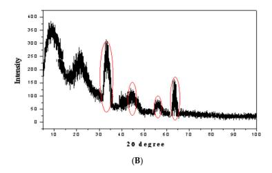
**Figure 4.** XRD spectrums of **(A)** amine-functionalized silica gel (ANSG) and **(B)** magnetic amine-functionalized silica gel (MANSG).
