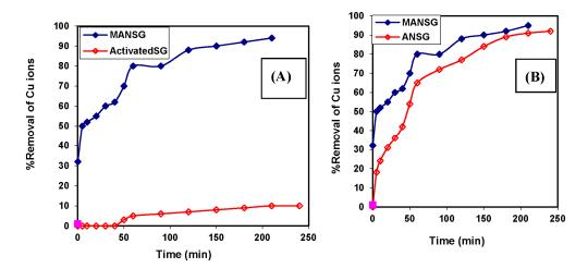
**Figure 9.** Comparable investigation of the influence of contact time on copper sorption process: (**A**) for both MANSG and its parent activated silica gel (Activated SG); (**B**) for both MANSG and its parent amine-functionalized nano-silica gel (ANSG). Solution concentration of ion = 1000 ppm; amount of adsorbent = 0.25 g; agitation speed = 200 rpm; solution volume = 25 mL; pH = 7.
