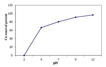
**Figure 12.** Effect of copper solution pH on the copper sorption process using MANSG (solution concentration of ion = 1000 ppm; amount of MANSG = 0.25 g; agitation speed = 200 rpm; solution volume = 25 mL; time = 90 min).
