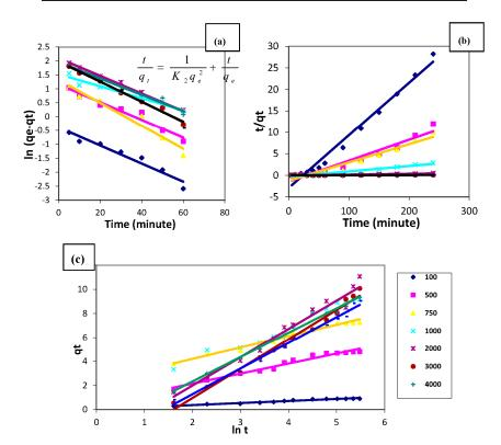
**Figure 16.** Kinetic models for the copper sorption process (solution temperature =  $25 \,^{\circ}$ C; amount of MANSG =  $0.25 \, \text{g}$ ; agitation speed =  $200 \, \text{rpm}$ ; solution volume =  $25 \, \text{mL}$ ; pH = 7): (a) pseudo-first-order rate model; (b) pseudo-second-order rate model; (c) the simple Elovich model.
