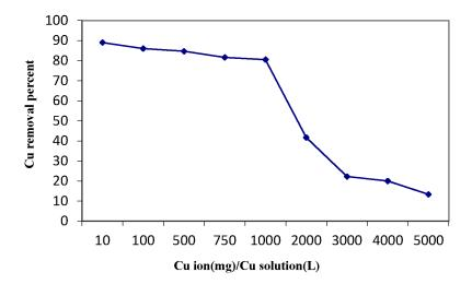
**Figure 11.** Effect of initial copper ion concentration on the copper sorption process using MANSG (time = 90 min; amount of MANSG = 0.25 g; agitation speed = 200 rpm; solution volume = 25 mL; pH = 7).
