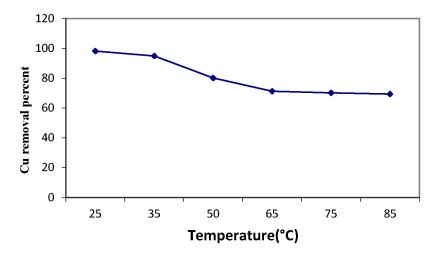
**Figure 13.** Effect of solution temperature on the copper sorption process using MANSG (solution concentration of ion = 1000 ppm; amount of MANSG = 0.25 g; agitation speed= 200 rpm; solution volume = 25 mL; pH = 7; time = 90 min).
