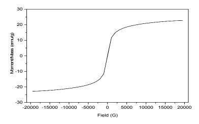
Figure 7. Isothermal M-H hysteresis curve of the magnetic amine-functionalized silica gel (MANSG).
