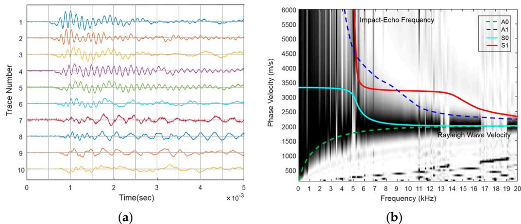
**Figure 8.** Experimental MASW results along Path III in specimen W2. The computed A0, A1, S0 and S1 Lamb modes corresponding to the specimen depth overlap on the dispersion curve image. (a) the signals in the time domain; (b) dispersion curve.
