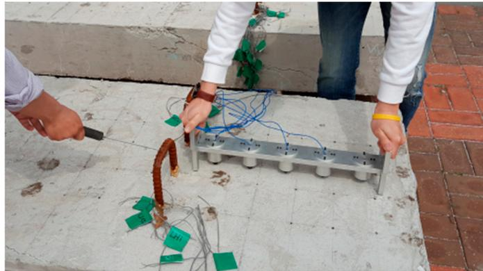
**Figure 7.** The MDAFS testing configuration for the MASW along predefined paths on the surface of a concrete wide beam.
