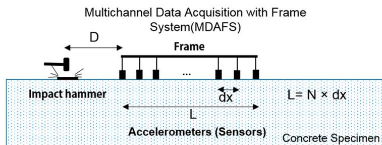
**Figure 4.** The scheme for an MASW test associated with MDAFS.  $D$  is near the offset;  $dx$  is the sensor spacing; and  $L$  is the offset range.
