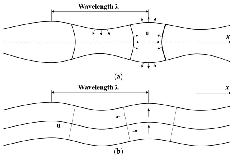
**Figure 2.** Mode shapes of symmetric (S0) and antisymmetric (A0) fundamental Lamb wave modes. (a) Symmetric mode; (b) antisymmetric mode.
