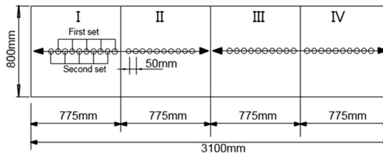
**Figure 6.** A planar view of the four test paths for the MASW test. The O marks indicate the sensor positions in each path, and the arrows show the direction of each test.
