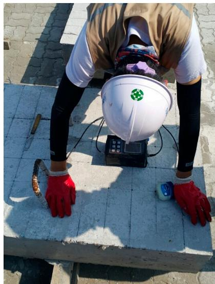
**Figure 9.** P-wave measurement in a grid on the surface of a concrete wide beam.
